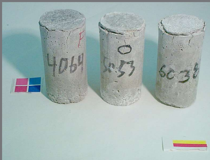
Cylinders exposed to \text{MgCl}_2 solution after 84 days of constant low temperature test. From left to right: 0.40, 0.50, and 0.60 w/c
