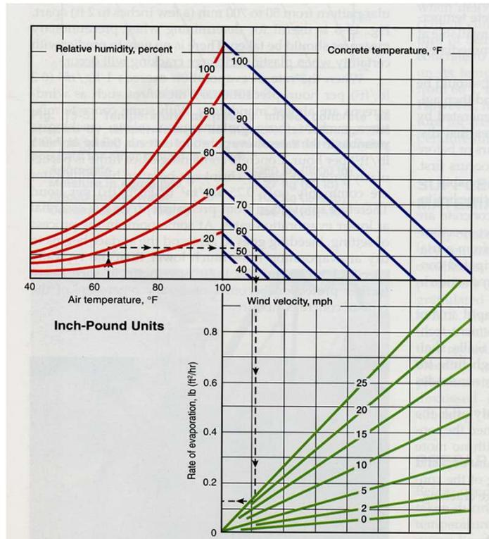
When the evaporation rate exceeds 0.2 lbs/ft<sup>2</sup>/hr precautionary measures are required to prevent plastic shrinkage cracks from forming.
