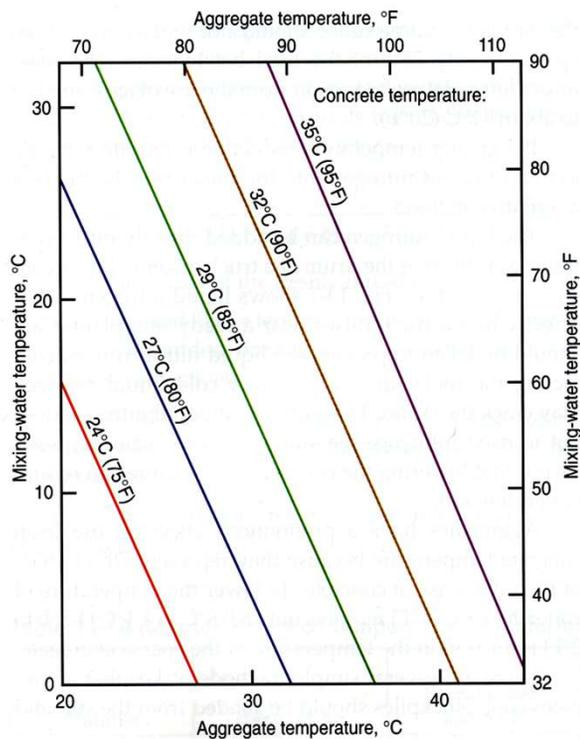
During hot weather conditions, keep aggregates and water as cool as possible.
