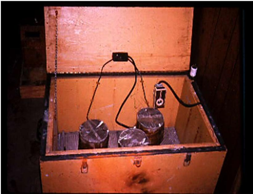
For specified compressive strengths less than 6000 psi, initial curing requires cylinders be stored at a temperature between 60-80°F for a period not exceeding 48 hrs.
