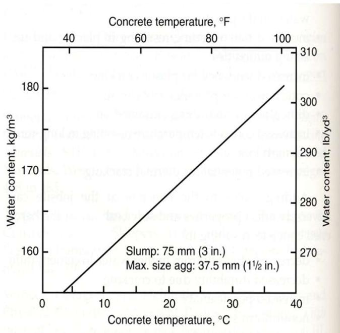
An increase in concrete temp results in an increase in water demand. From 50-100°F, 33 lb/yd<sup>3</sup> of additional water is needed to maintain a constant 3 inch slump.
