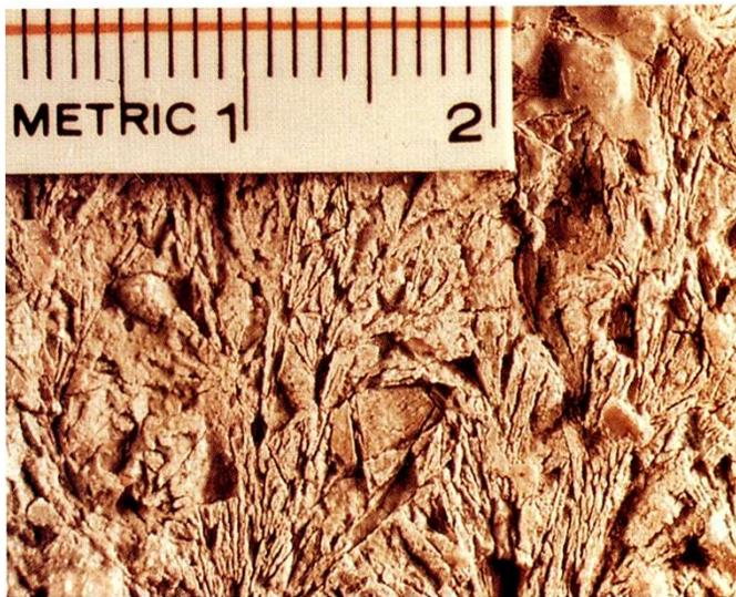
Concrete that has froze just once at an early age can be restored to **nearly** normal strengths by providing a proper curing environment. Such concrete, however, will not be as resistant to weathering nor as impermeable as concrete that had not froze.
