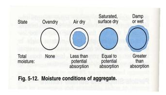
Aggregates have an internal void or pore structure that at any time may or may not contain water (absorbed water). Depending on the moisture content, the four possible conditions for aggregates are as follows:
